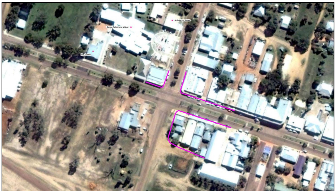
Figure 4: Indicative alignment of CBD mobile flood barrier
