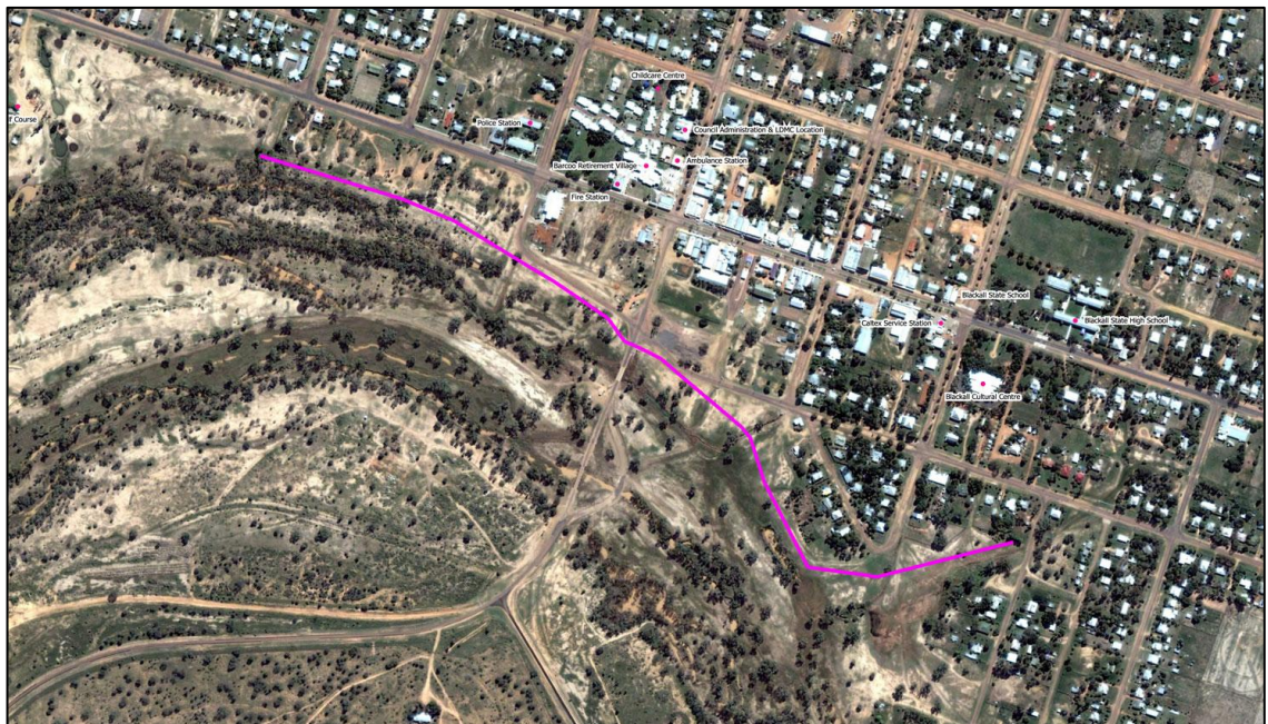
Figure 3: Indicative alignment of permanent CBD levee
